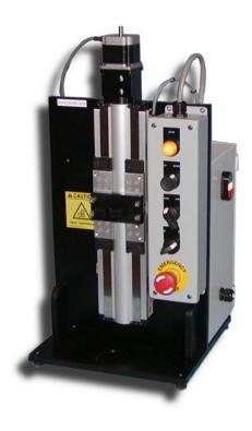
AVID Innovation's DIP200 Dipping Station enables automatic control of the dip rates and depth of a medical device into a chemical solution.
